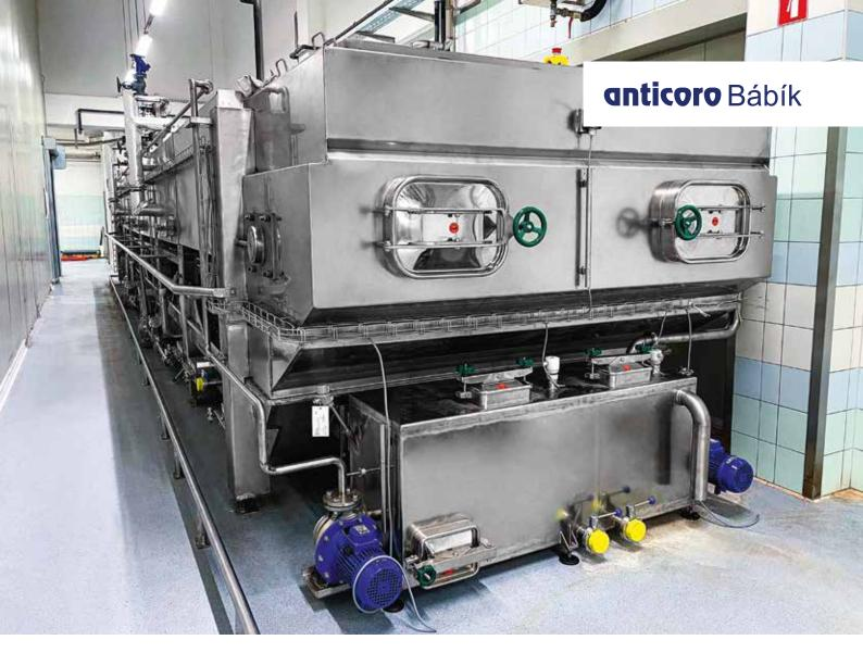
*Construction of Tofu pasteurizer is very robust, all stainless steel. Partial thermal insulation reduces the thermal energy consumption.*
